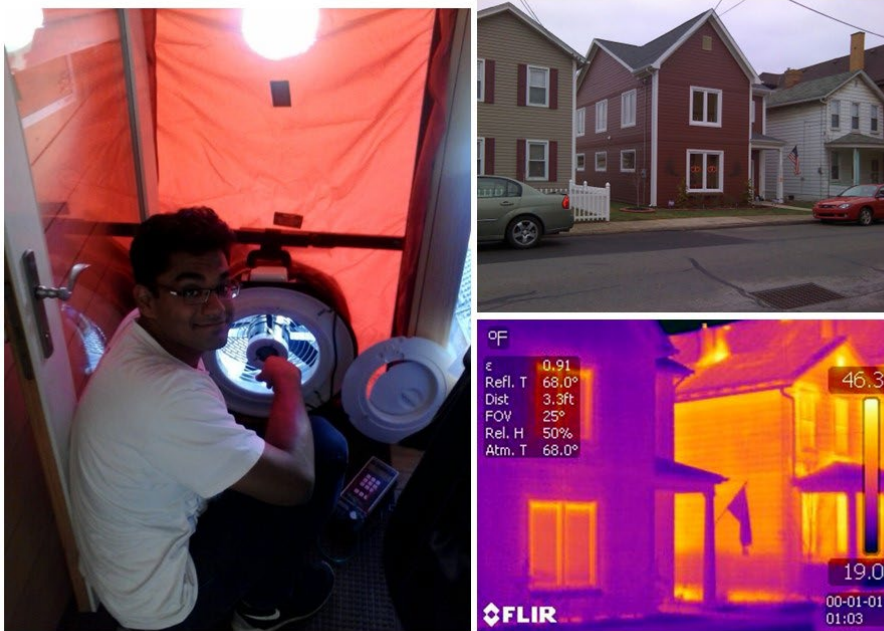
Caption: Infrared images reveal envelope performance and CMU grad, Ashwin Ranna, prepares for blower door test. Photo credit: N Baird
