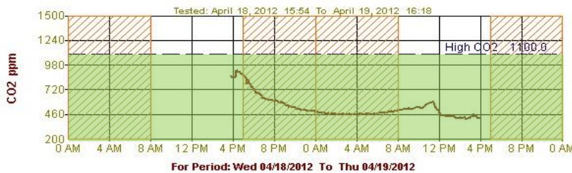
Figure 24 Continuous measurement result: CO2 concentration
