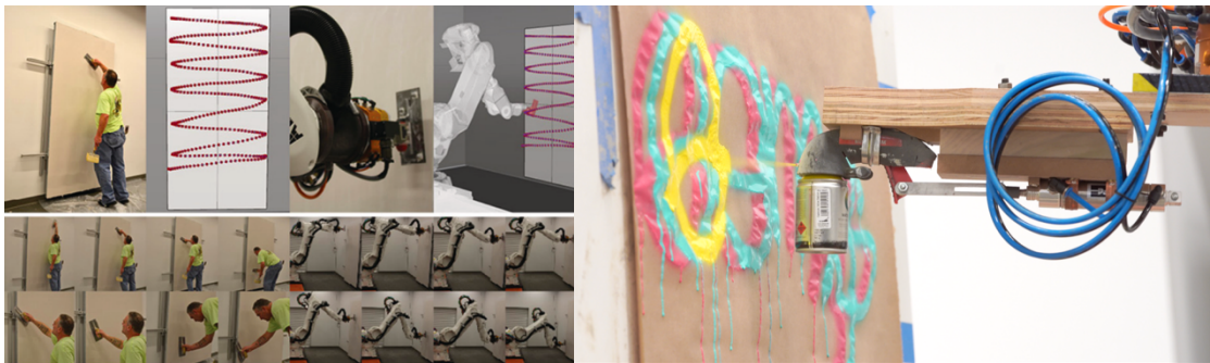
Figure 5- Robotic plastering (left) and graffiti (right) (Bard et al. 2014).
