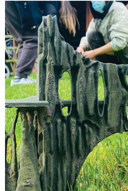
Lithopic House Studio (2021): Physical prototype of facade system, model developed from image texture into computational model and 3-d printed from sand (Student: Juhi Dhanesha)
