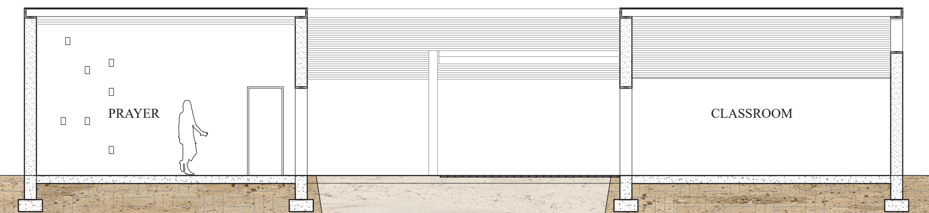
WALL SECTION: RAMMED EARTH 1/2" = 1'0"
